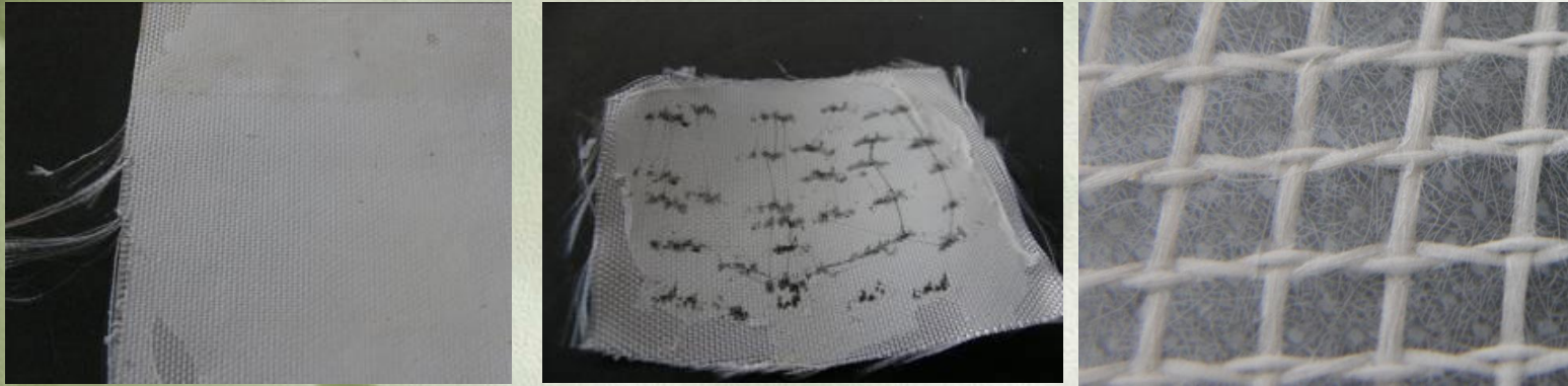
Fig.: Tests of bonding of PI nanofiber layer on the glass fabric substrate
