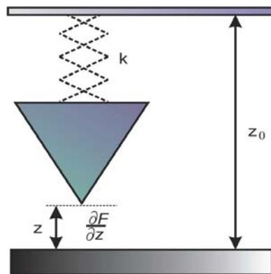
**Fig. 2** Modeled tip-sample interaction, where  $k$  denotes cantilever constant and the force derivative  $\partial F / \partial z$  is schematically depicted here as an additive force interaction constant.
