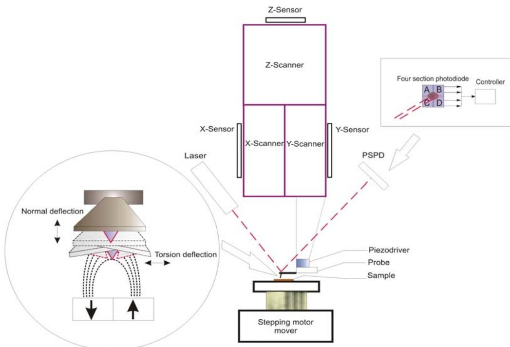
**Fig. 1** MFM block controller scheme. The laser beam is focused on the flexible cantilever. While the cantilever feels any stray field changes, the angle of the deflected light changes as well. Reflected light is registered by sensitive detector (four section photodiode PSPD) and transformed to the electric signal (organization known as the optical lever set-up).
