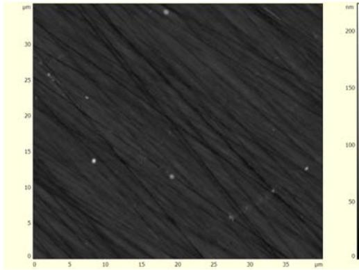
**Fig. 3** First pass: surface topography imaging - semi-contact or tapping mode (magnetic recording medium).
