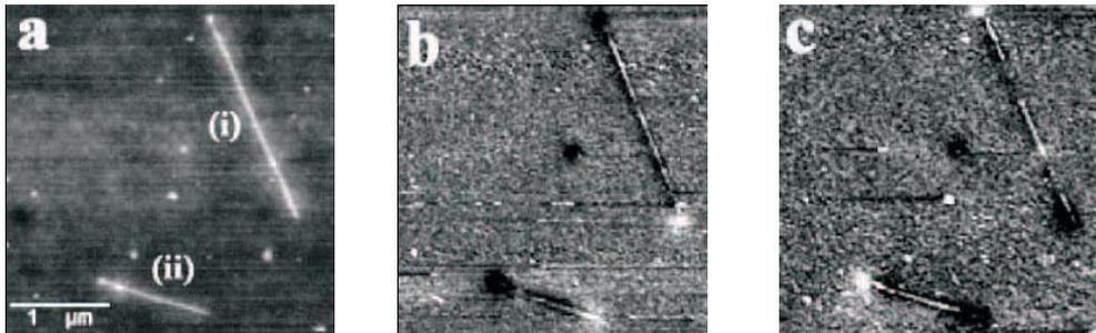
**Fig. 5**  $\text{Fe}_3\text{B}$  nanowire image obtained by AFM (a) and the same image obtained by MFM (b). The last image was performed by MFM after the reversion of tip magnetization. The change of magnetization is depicted by alternating bright and dark nanowire ends (reprinted from ref. [20]).
