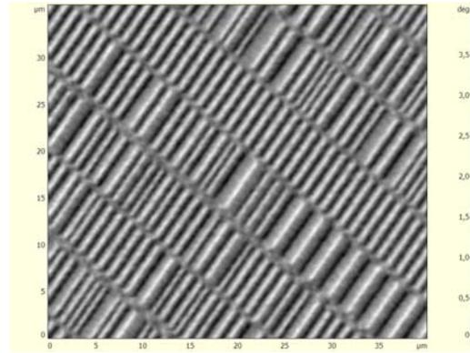
**Fig. 4** Second pass: lift scan follows the topography to obtain magnetic contrast image (magnetic recording medium).
